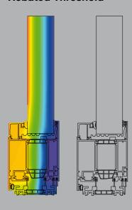
The 5-35D Hi and 5-35D Hi+ systems offer significantly improved U-frame values over more traditional, thermally broken, aluminium door systems.
